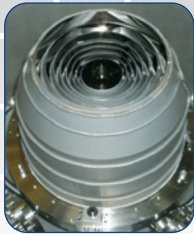
Wolter Grazing Incidence Collector
